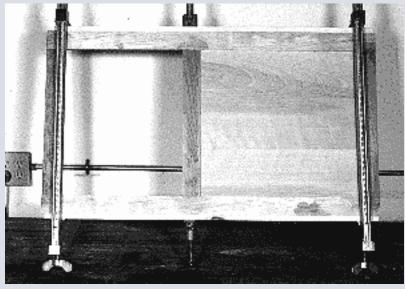
Photo 2- Glue together the side frames as shown. Check them for square and adjust as necessary.
