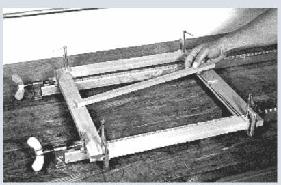
Photo 3- Join the drawer frames with groove and tenon joints cut at the table saw, then glue them up as shown. Install drawer guides in the front and rear pieces.
