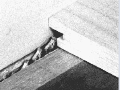
Photo 8- The second step in cutting the joints on the drawer fronts is to shorten one of the tongues.
