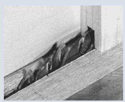
Photo 7- The first step in cutting the joints on the drawer fronts is to make this vertical cut on end. Note that you can do the same for the drawer rears, or just fit them into dadoes in the sides that are set 1" ahead of the rear end of the sides.
